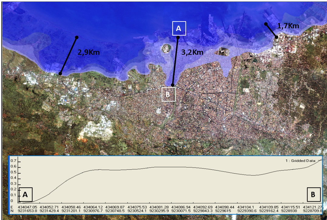
Figure 2.8 (b): Sea Water Inundation in Semarang City in the Next 100 Years with SLR Estimation at 80 cm
