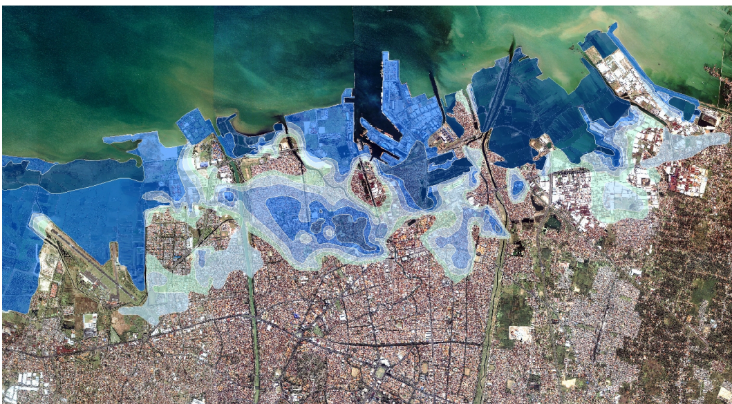
Figure 2.8 (a): Sea Water Inundation in Semarang City in The Next 100 Years with SLR Estimation at 80 cm
